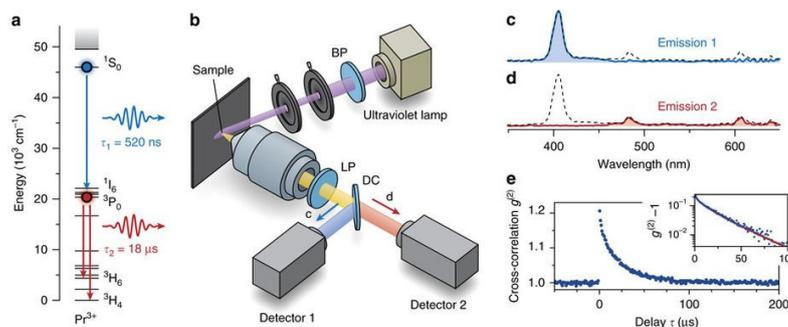
Figure 1 – Illustration correlated photon counting to demonstrate two-photon emission using NaLaF<sub>4</sub>:Pr<sup>3+</sup> as model system. (a) Two-photon emission on Pr<sup>3+</sup>. (b) Schematic set-up for correlated photon counting (c, d) Emission of Pr<sup>3+</sup> in blue and red spectral region detected by separate detectors. (e) Correlated photon-counting signal.
