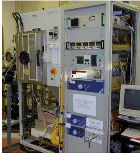
Figure 2.3: Magnetron sputtering preparation chamber at the ICMM
